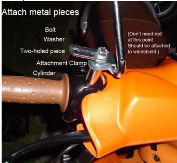
Also note that, as pointed out by others, the right hand, reverse-thread bolt might be too long. As James Tate recommended, you might want "six or so washers just to be sure you don't bottom out and damage the housing you are screwing into. Make sure to put them above the metal clamp so the height of the shield arm stays the same."
