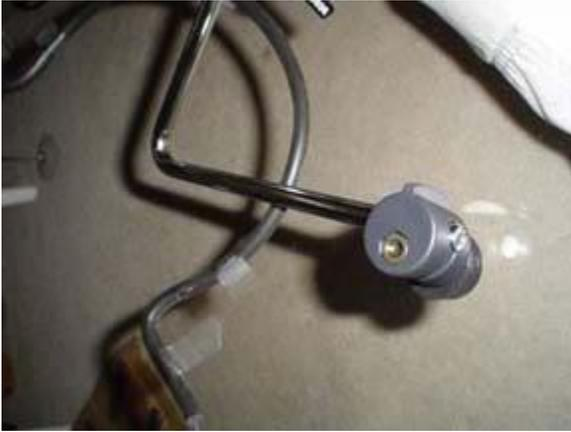
5. Remove the mirrors from the scooter. They just twist off, but note that the right-hand side is reverse threaded!
