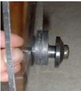
3. Add the black rubber piece that will attach the windshield to the metal rod. (The skinny hole goes closest to the windshield so that the nut can screw onto the back, the screws go to the outside and the rubber nodule thing to the inside.)
