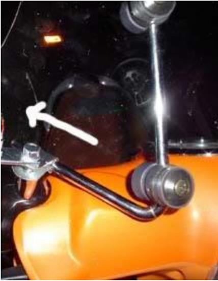
9. Make sure it is on straight. Easiest way to tell is by looking at the area around the headlight and making sure it is even all the way around. Then hold in place and tighten the bolts, but don't make them immovable yet.
