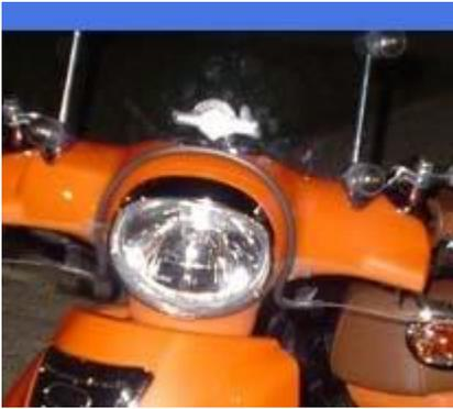
10. Bolt the mirrors on and adjust as needed. Again remember the right hand side is reverse threaded.
